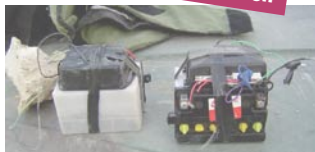
A battery and car alarm system used as a remote control detonator.
