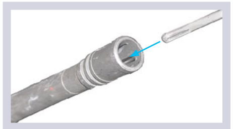
Shove rod into barrel to clear jammed cartridge.
