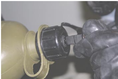
Carefully connect drinking tube.
